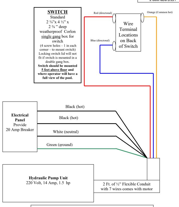
After final wiring, if the cover movement doesn't agree with the "Cover" – "Uncover" labels on the front of the switch, just reverse the positions of the red and blue wires on the switch.
